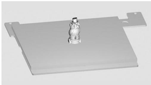
3. The second part will open in the center of the bed and appear to be merged with the first part.
