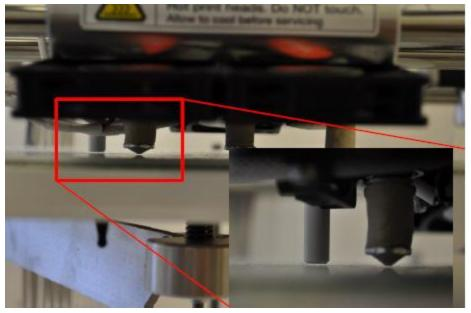
Once your Wiping Stick is properly aligned to the Print Tips you will need to lock it back in place. This is done by holding the Wiping Stick bolt in place with the 2.5mm hex driver and turning the bolt with the 3mm wrench until is locked against the wiping stick fastener.
