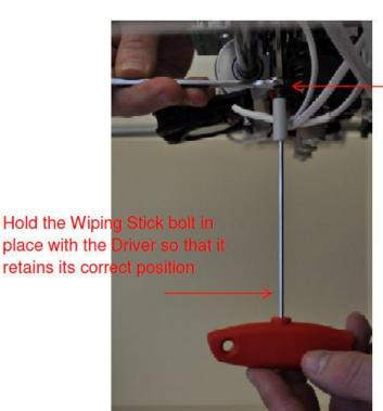
Lock The nut against the Wiping stick fastener with the M3 spanner
