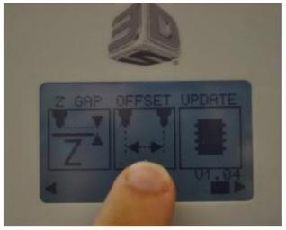
The Wiping Stick offset needs to be set so that the stick will just touch the Jet Wiper as it moves past it. if it is too far behind the wiper it will not clean the wiper efficiently. If too much of the wiping stick hits the wiper it can cause printing problems such as shift in parts or in extreme cases damage to the CubeX.
