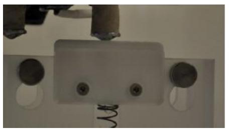
This is the height of the jet wiper relative to the Print Tip. This setting ensures all waste is correctly wiped from the Print Tip
