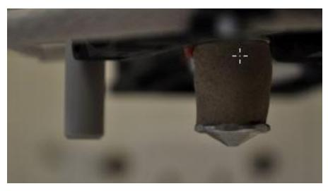
This is the Wiping stick height relative to the Print Tip. This setting ensures that all waste is knocked from the Jet Wipe and into the waste collection bin.
