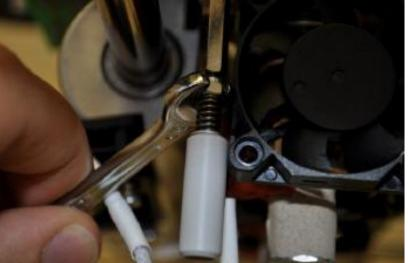
Holding the Nut in place with the 3mm wrench, use a 2.5mm hex driver to adjust the wiping stick bolt. Turning the driver clockwise will lower the wiping stick height and turning it anti-clockwise will raise the wiping stick height.
