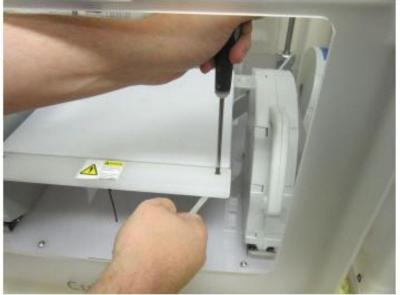
4. Once both bolts are loose on the stabilizer bar, push the bar towards the back of the printer and tighten the bolts.
