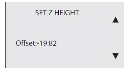
2. Using the “Down” arrow, lower the print pad down by 0.1 from the print jet tip. Click on the Control button, the next screen will allow you to save the setting. Click on the check mark to save or the X to cancel the setting.
