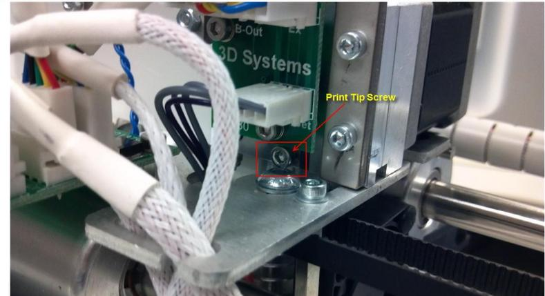
4. Turn the Z-axis drive screw by hand clockwise to raise the Print Pad up until the print tips all touch the Print Pad and are aligned with each other. (Note: The Z-axis drive screw will likely have a thin coating of grease; use gloves or protect your hand with a paper towel if this is a concern)
